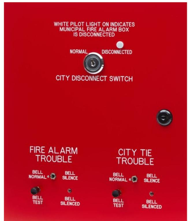
The City Tie Disconnect Panel operates on 24VDC. It comes wired with a negative common, positive is available upon request. The panel can also have a module used to disconnect the City Tie if requested.
