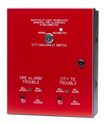
The City Tie Disconnect Switch is used to disconnect the Fire Alarm Panel from reporting any Alarm or Trouble condition to the city in order to test and maintain the Fire Alarm System. When the switch is turned to the DISCONNECTED position, a white pilot light illuminates which informs the user that the Panel has been disconnected. The City Tie Trouble Bell will ring and can be silenced using the City Tie Trouble Station to the right of the Disconnect Switch.
